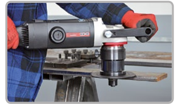
Steel plate beveling
