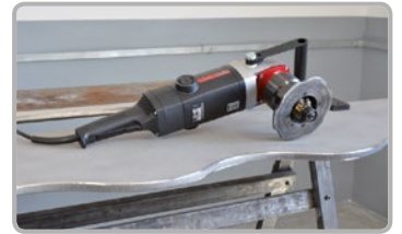
Arched edge beveling with radius
